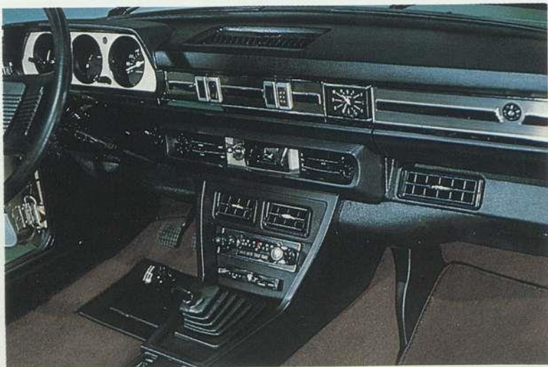
Directional air conditioning ducts are strategically spaced across the dash.
