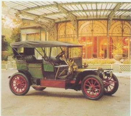
The 1906 chain-driven Torpedo, powered by an advanced four-cylinder, 12 horsepower engine.
