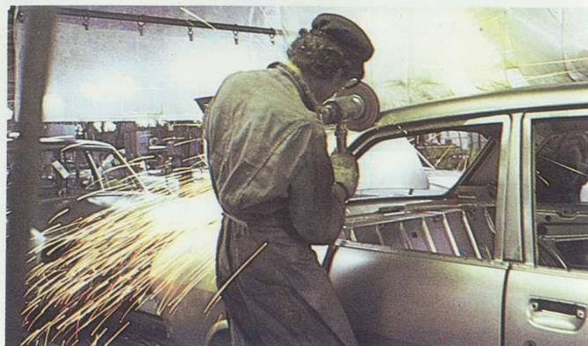
Every welded seam is sanded smooth so you can't see it.
