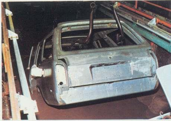
Every Peugeot is dunked in an electrophoresis primer bath.
