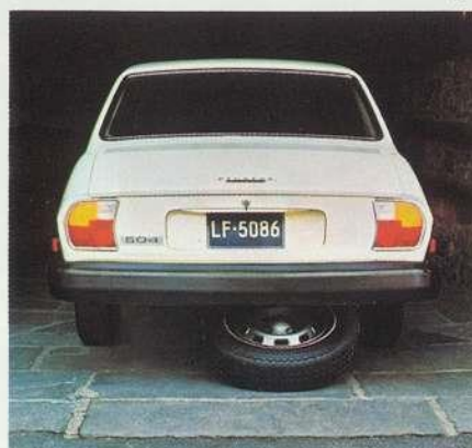
The spare tire is mounted under the car.
