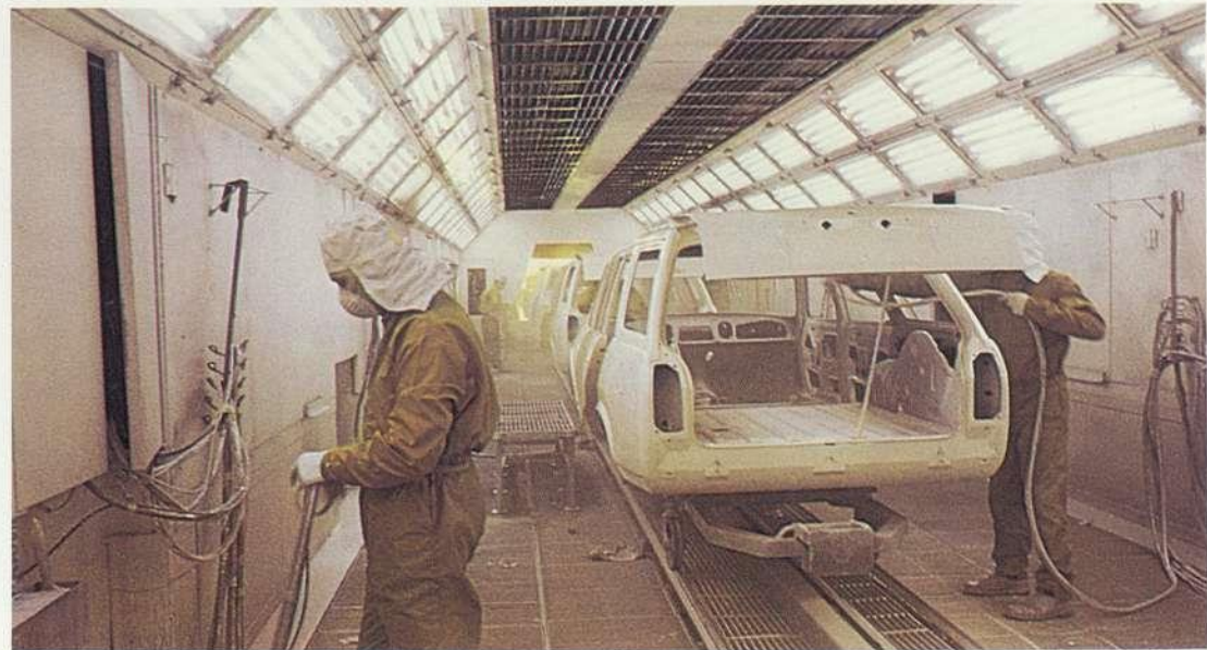
Each car gets a six stage protective finish. The last two coats are sprayed on by hand and baked in an infra-red oven.
