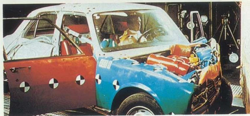
The entire crash is filmed in slow motion and each car is carefully studied. Above, a front-angle crash.
