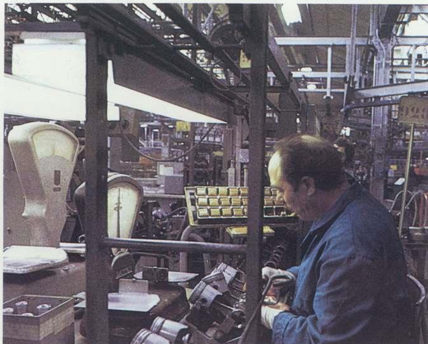
Pistons are carefully matched and weighed for each engine to achieve near perfect balance.
