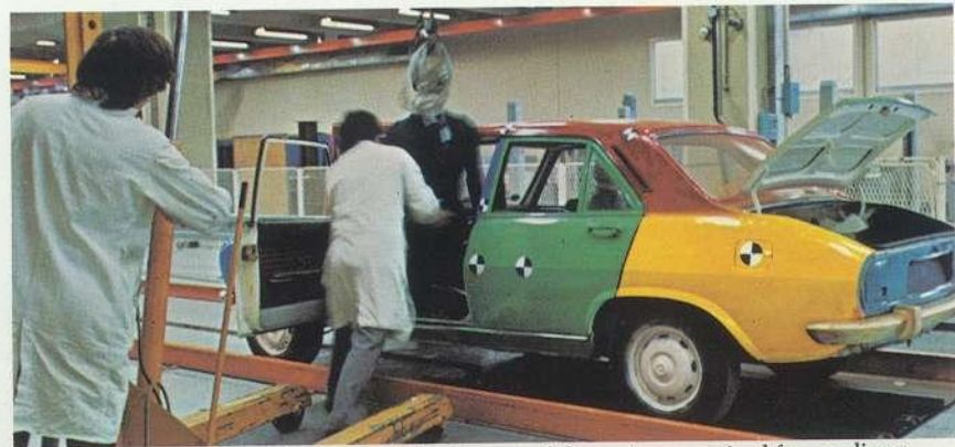
At the beginning of a test crash both car and dummies are wired for readings.
