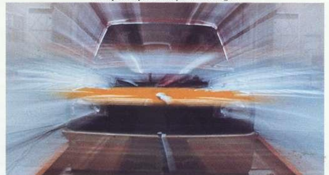
Then the car is either catapulted or driven into a concrete barrier.
