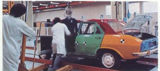
The beginning of a test crash: Both the car and the dummies are completely wired for readings.
