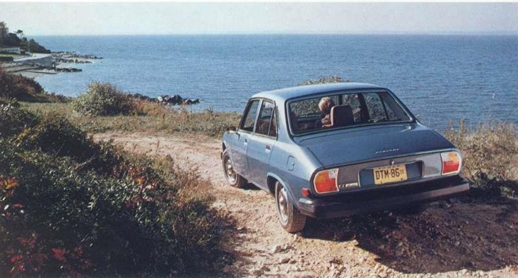
The 504 gives you a superb ride on almost any kind of road. Some of the reasons: 4-wheel independent suspension, shock absorbers with unusually long travel, and front and rear anti-sway bars.
