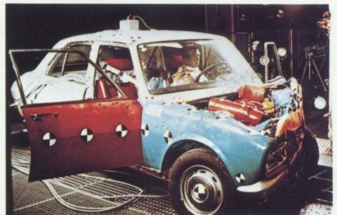
The entire crash is filmed in slow motion and each car is carefully studied. Above, a front-angle crash.
