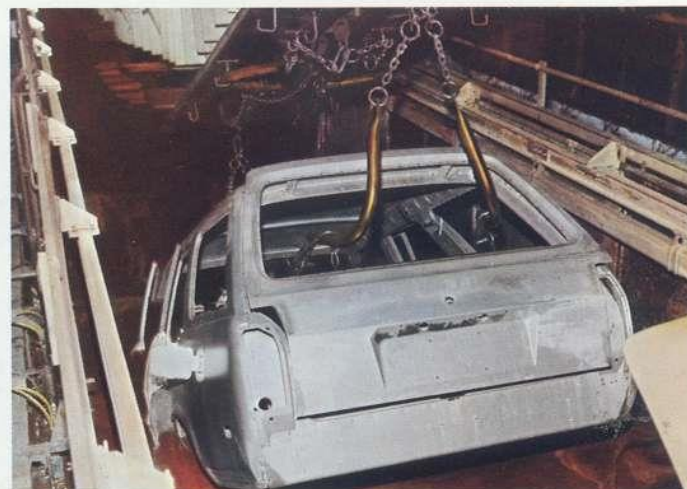
Every Peugeot is dunked in an electrophoresis primer bath to deter rust and corrosion.
