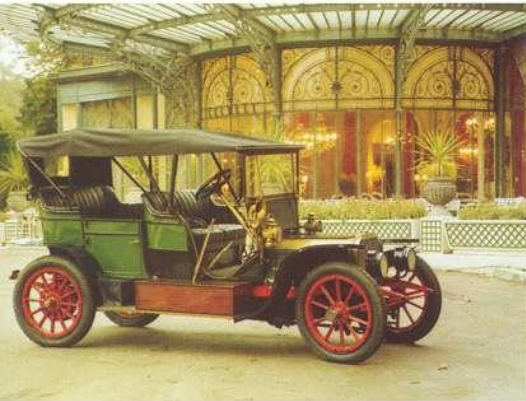
The 1906 chain-driven Torpedo, powered by an advanced four-cylinder, 12 horsepower engine.
