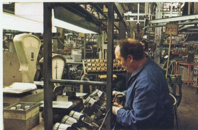
Pistons are carefully matched and weighed for each engine to achieve near perfect balance.
