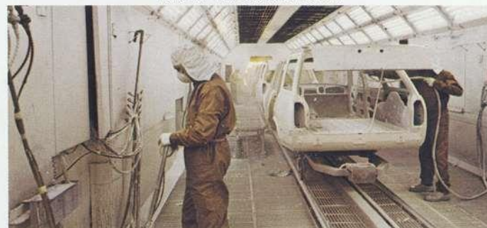
Each car gets five coats of protective finish. The last two coats are sprayed on by hand, then baked in an infra-red oven.
