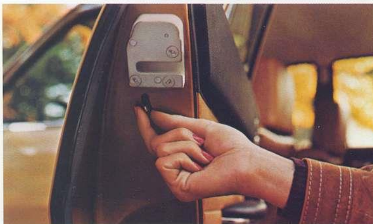
Child-proof door locks let you open the rear doors from the outside, but not from the inside.
