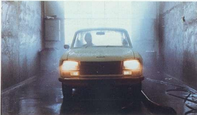
A Peugeot is tested for water leaks in a special chamber that simulates a rain storm at high speed.
