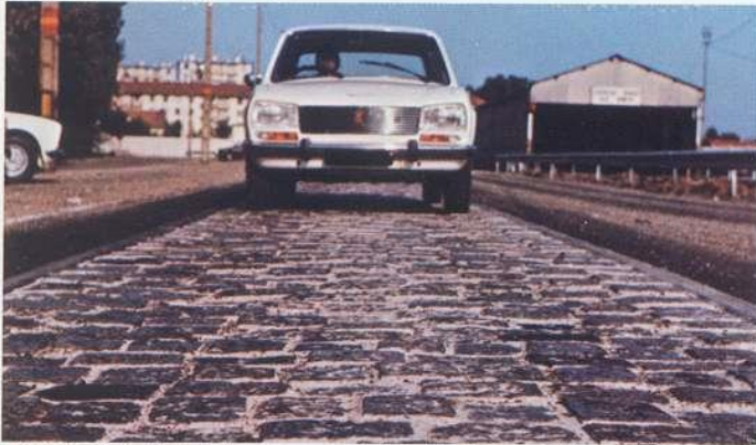
Each car is then taken on a special test track to make sure there are no rattles and to check ride and handling.
