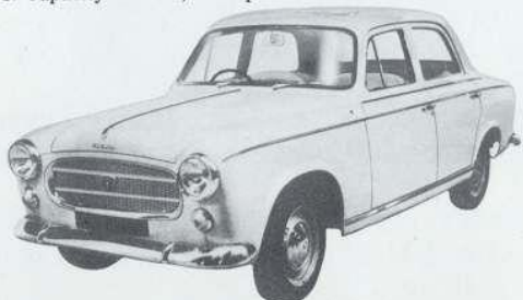
Peugeot 403 (1955-1966). A big jump in styling and comfort from the 203, with a similar jump in engine capacity and power — up to 1468 cc and 65 bhp.
