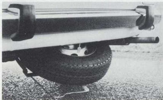
Spare wheel cradle released via catch in boot compartment.
