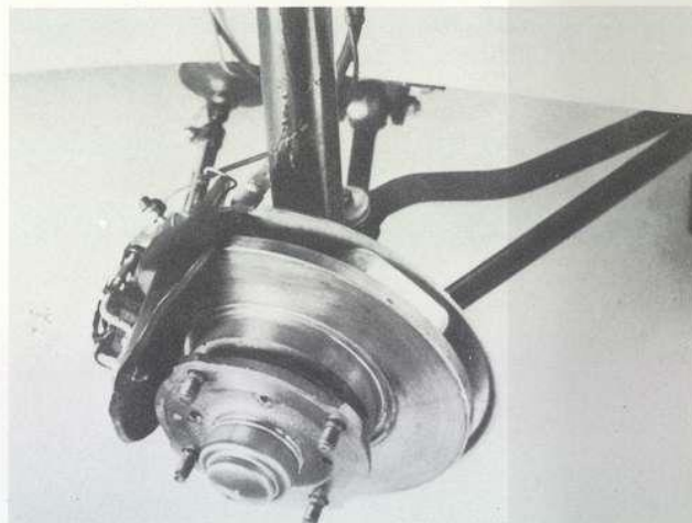
Dual circuit, power-assisted disc brakes on all four wheels.
