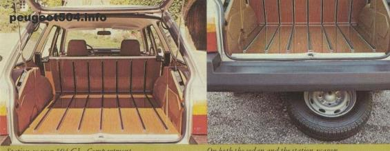
Station-wagon 504 GL. Compartment capacity: rear seat in upright position 41.34 cu. ft.; rear seat in down position 67.13 cu. ft.
