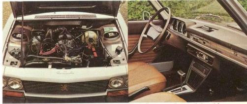
4 cylinder, 2 liter engine with 2 single barrel carbs; overhead valves; 92 hp at 5600 rpm. Top speed 105 mph; cruising speed 85 mph; plus European style gas consumption.
