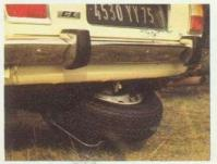
Large boot, a total luggage volume of 19.3 cu. ft. with automatic boot light. Spare wheel housed in an independent cradle located beneath the boot, locked from the interior.
