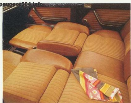
The adjustable front seats recline fully to form twin couchettes. Automatic interior lighting on the opening of the doors by two side bracket lights.
