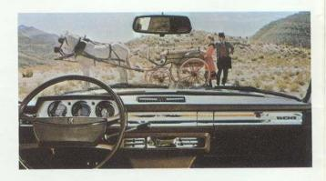
Padded, anti-reflective safety dashboard. Lockable glove box and automatic interior lighting. Supplementary storage shelf.
