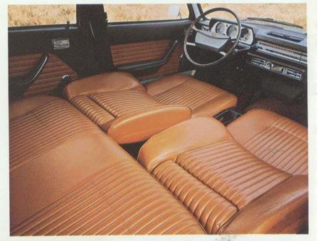
The front seats are adjustable and recline fully to form twin couchettes. Thick carpets fitted at front and rear.
