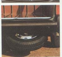
Dashboard with three round dials incorporating electric clock. Spare wheel housed in an independent cradle located beneath the boot.
