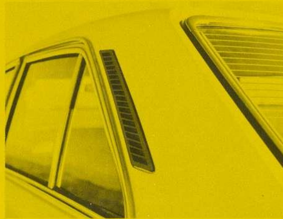
Large "flow-through" ventilation outlets clear interior air, keep it circulating, fresh. Electrically heated rear window promptly clears away condensation.
