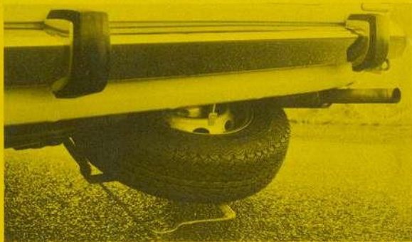
To achieve more usable luggage space and give easier access to the spare, Peugeot designers have placed the wheel under the boot, from where it is simply released by a catch located at the rear of the boot compartment.
