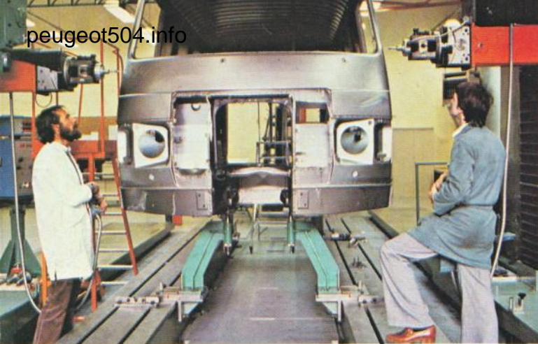
Machine à mesurer (Usine de Gennevilliers) Body measuring machine (Gennevilliers plant) Mess-Maschine (Gennevilliers Werk)
