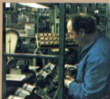
Pistons are weighed for near perfect balancing.
