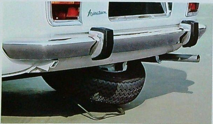
The spare-wheel is mounted under the floor thereby ensuring maximum loading space in the luggage boot.
