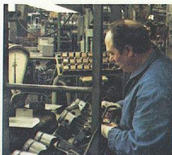
Pistons are weighed for near perfect balancing.
