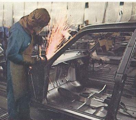
Every welded seam is sanded smooth so you can't see it.
