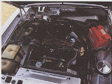
3235cc V6 provides 165bhp but car still feels underpowered. Sounds good though
