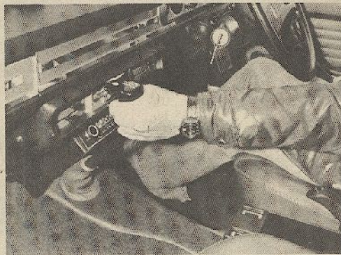
Above: floppy gearchange due to missing linkage bolt. Above right: the original seat belts were replaced under warranty because of sticking reels. Below left: lights stalk too close to steering wheel. Below right: both front door striker plates worked loose
