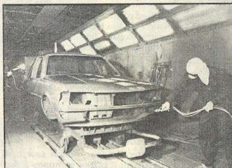
Above: Centre for the 104 model is the plant at Mulhouse. Below: Paint spraying for the new 305, and assembly at the ever-interesting stage where the body meets its machinery. The engine is an all-aluminium structure. Right: Final approach for crash test
