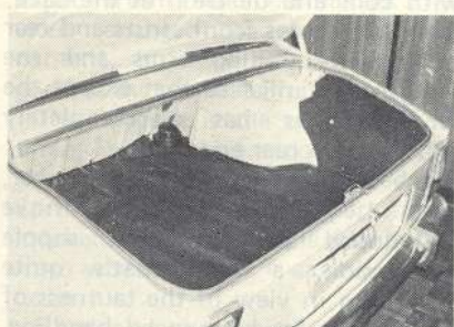
ALFETTA (left) has a fully-lined boot, the Sprint's area (centre) is too shallow, while the Peugeot (right) is biggest of the three. Alfa and Sprint spares hide under the mat, Peugeot stores its wheel in a sling under the car.
