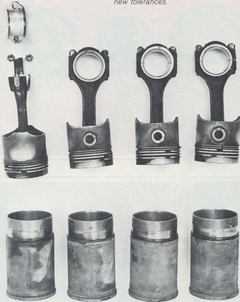
Piston assemblies, wet-sleeve cylinders barely showed signs of use, and in most critical areas retained new tolerances.
