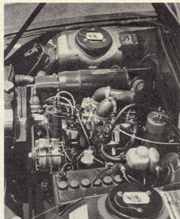
Peugeot's engine is slant-mounted.
