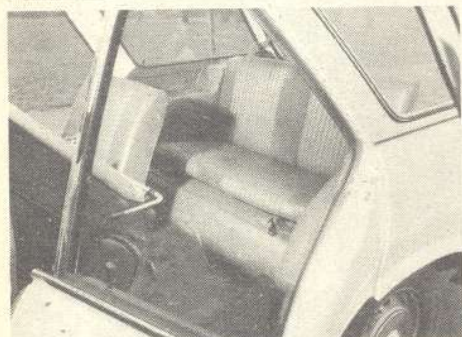
The seats get progressively higher and less comfortable from front to back. The front ones, right, are excellent — deep, fully adjustable armchairs with built-in headrests (pushed in here). The centre row, below, are good, those at the back, above, unshaped and rather hard
