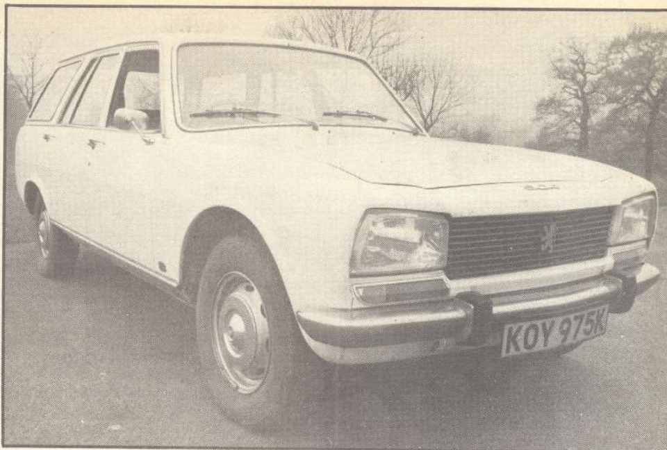
Below: the long rear overhang and stepped roof — to increase headroom and rigidity — emphasize the car's near-16ft. length, though we find the styling well proportioned. The aim of the headlights, above, can be adjusted. Massive rubber-faced overriders protect against clumsy parkers. The rear window, right, soon becomes opaque with dirty spray in wet weather
