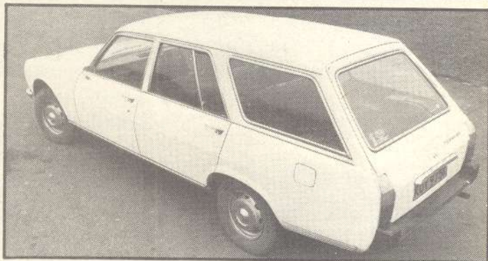
Below: the long rear overhang and stepped roof — to increase headroom and rigidity — emphasize the car's near-16ft. length, though we find the styling well proportioned. The aim of the headlights, above, can be adjusted. Massive rubber-faced overriders protect against clumsy parkers. The rear window, right, soon becomes opaque with dirty spray in wet weather
