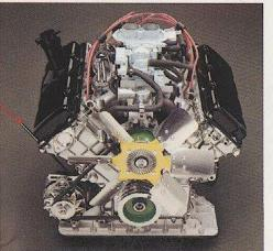
Six cylinders in 90°V -Oversquare - Aluminium cylinder block - Removable wet cylinder sleeves - Aluminium cylinder heads with hemispherical chambers -Overhead camshaft per bank of cylinders - Four-bearing crankshaft - Viscous coupled
