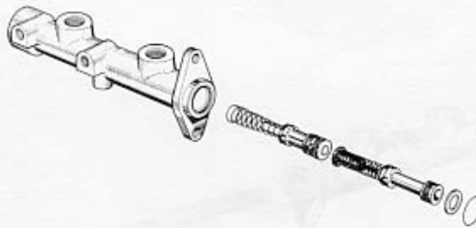
7 - For Lockheed master-cylinder, 19 m/m dia., travel 35 m/m (grooved a).
