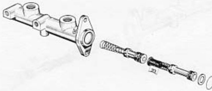
6 - For Teves master-cylinder, 20,6 m/m dia., 35 m/m travel. (numbered 20).
