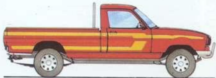
ADAPTATION 4x4 "DANGEL" sur base 504 Pick-Up Entrepreneur ou 504 Pick-Up Confort
