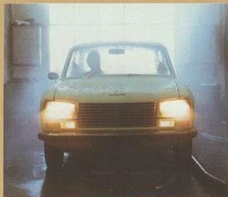
Each car undergoes a rain tunnel test for leaks.
