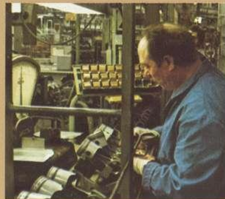
Pistons are weighed for near perfect balancing.
